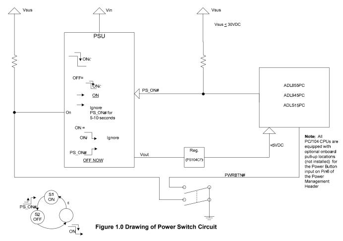
**NOTE:** Figure 1.0 depicts a simple external switch circuit that can be used to allow the user to power up the ADLxxxPC board by way of a single switch. Due to space limitations found in embedded form factors, this small circuit is often omitted from embedded designs.
