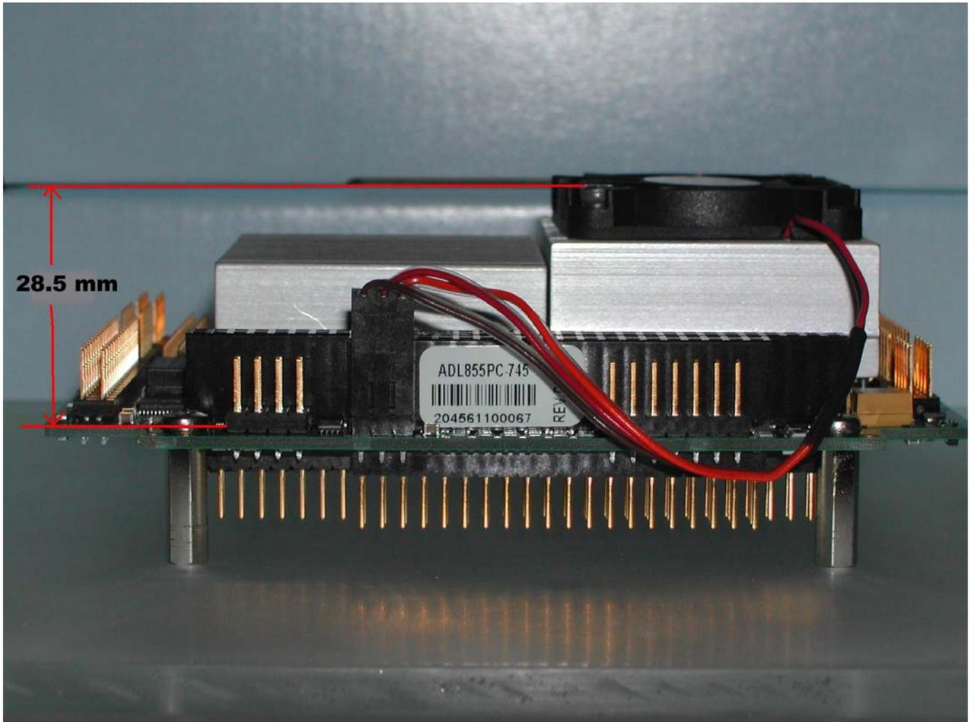
The two piece Heat Sink Solution was developed to offer a low cost high performance solution to customers that have the physical envelope for this implementation.
