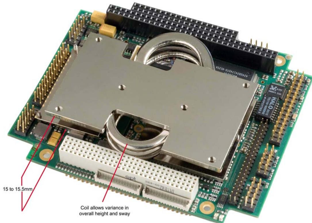
The ADL Embedded Solutions Heat Pipe Solution offers a very unique solution for customers who are concerned with overall weight of the thermal solution. It also provides the advantage of a very fast thermal response. The floating tip plate will accommodate small variances in surface mounting.
