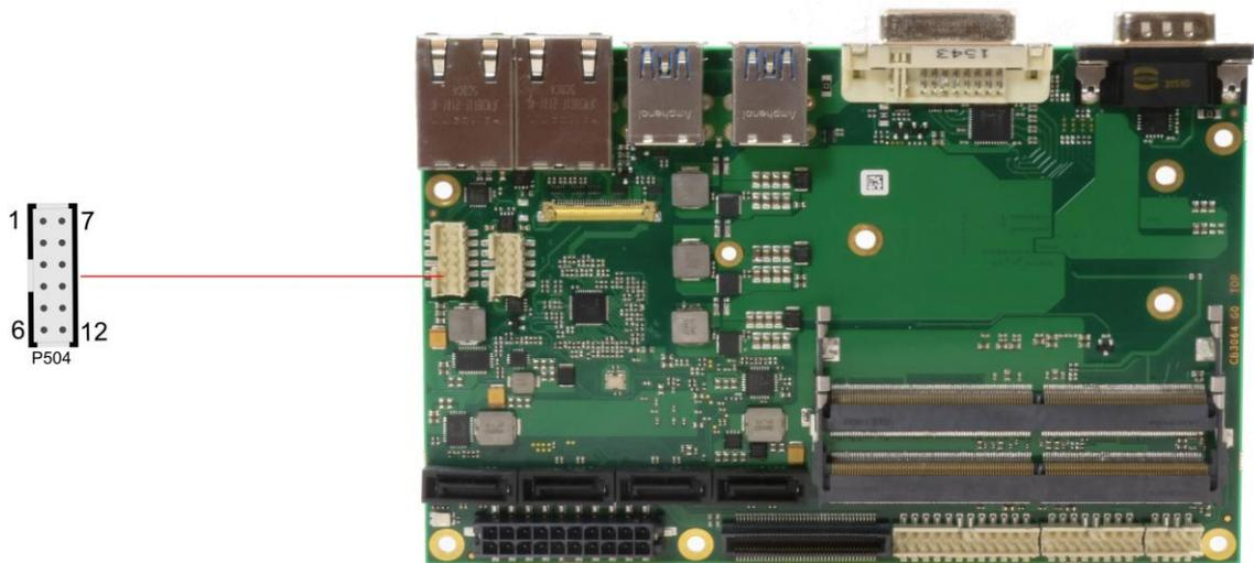
Pinout GPIO connector:
