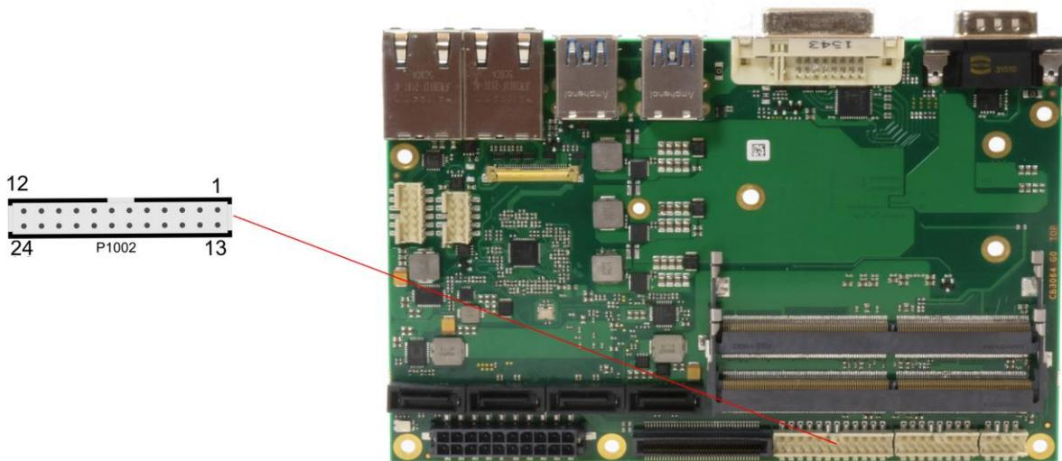
Pinout 2x12-pin connector:
