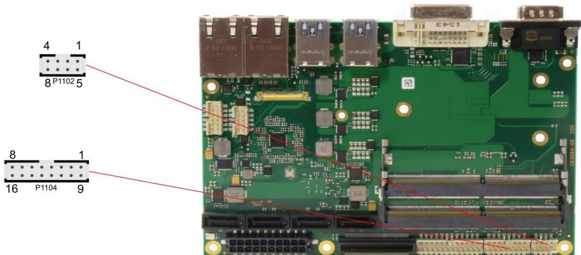
Pinout 2x8-pin USB connector:
