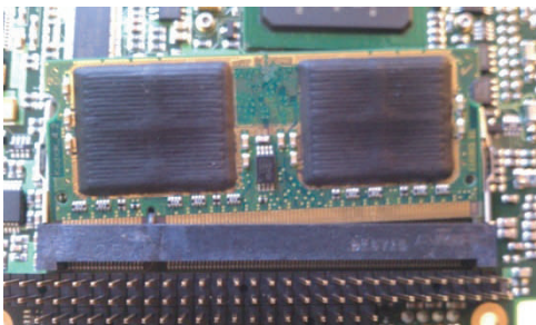
Figure 5) DDR-RAM loose but still in socket
